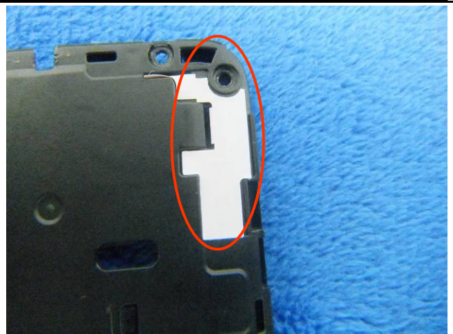
WIFI/BT/BLE/GPS - Antenna View
