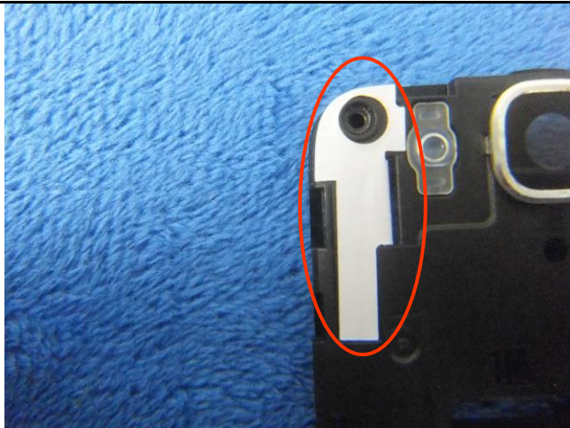
LTE Antenna View
