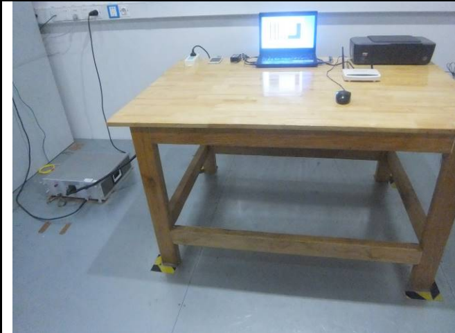
Conducted Emissions Test Setup – Front View
