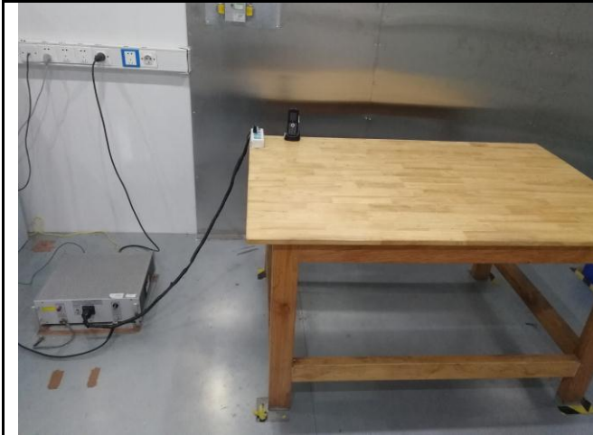
Conducted Emissions Test Setup – Front View
