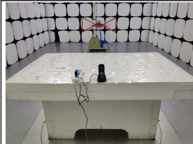
Radiated Emissions Test Setup Below 1GHz
