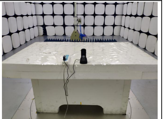
Radiated Emissions Test Setup Above 1GHz
