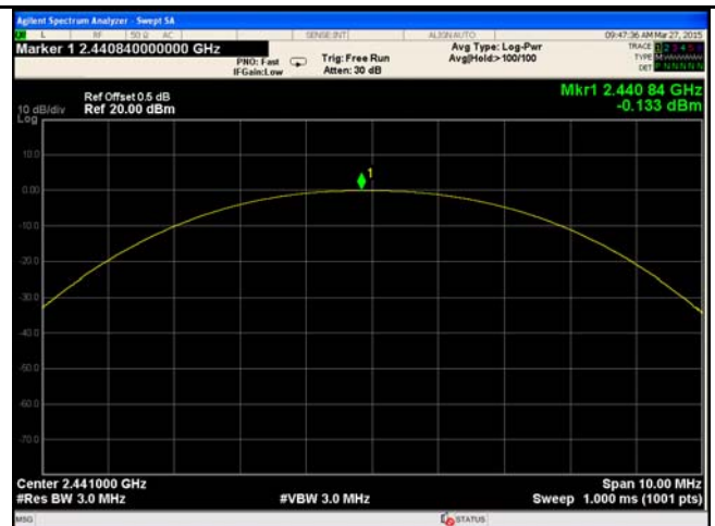
GFSK Output power - Mid CH 2441
