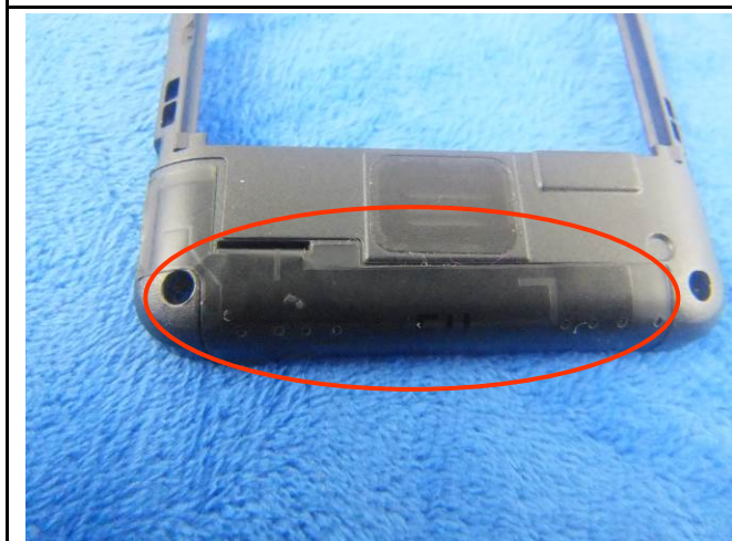
GSM/PCS/UMTS-FDD Antenna View
