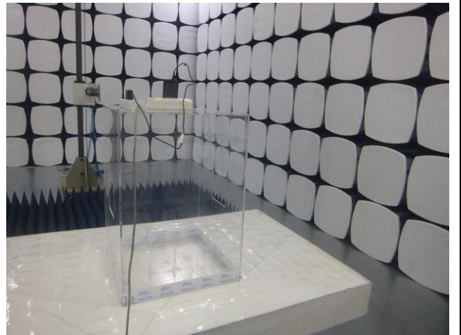
Radiated Spurious Emissions Test Setup Above 1GHz
