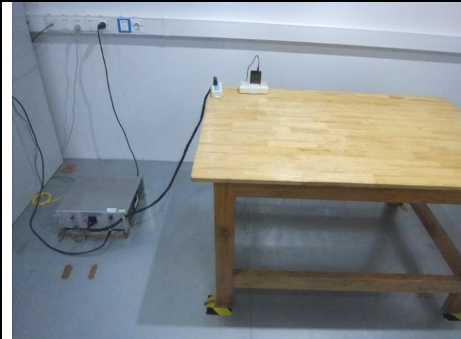
Conducted Emissions Test Setup Front View
