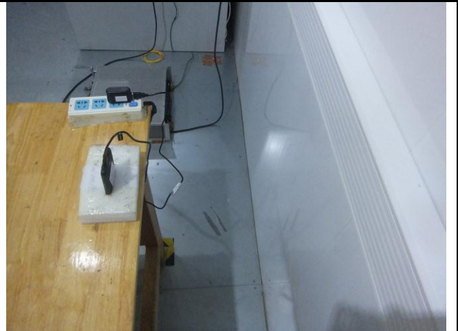
Conducted Emissions Test Setup Side View
