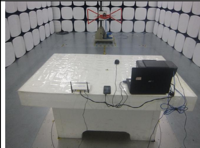
Radiated Emissions Test Setup Below 1GHz
