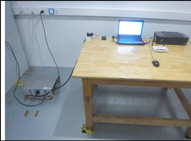
Conducted Emissions Test Setup – Front View
