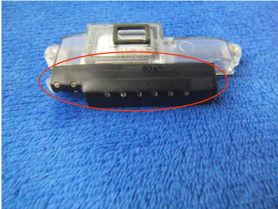
GSM/PCS/UMTS-FDD Antenna View
