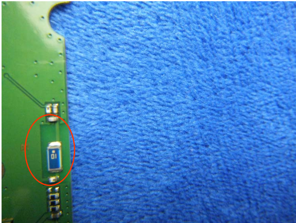
BT - Antenna View
