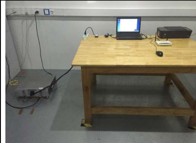
Conducted Emissions Test Setup – Front View
