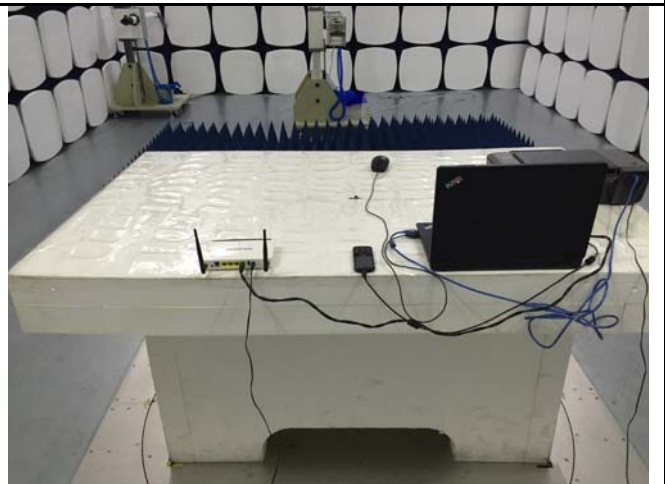
Radiated Emissions Test Setup Above 1GHz
