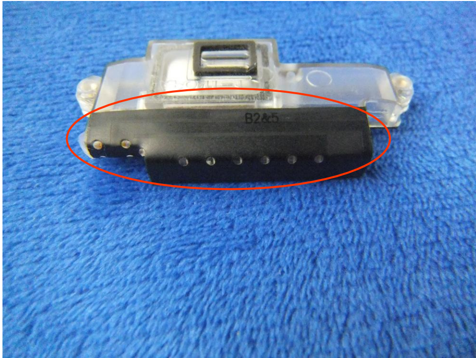
GSM/PCS/UMTS-FDD Antenna View
