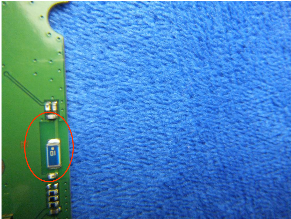
BT - Antenna View
