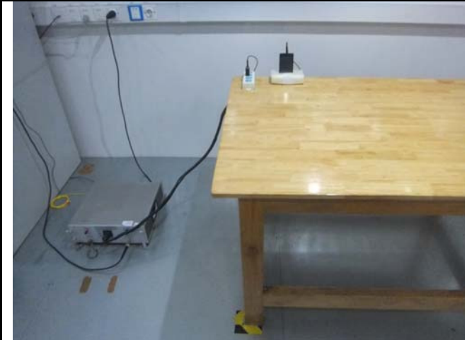
Conducted Emissions Test Setup Front View
