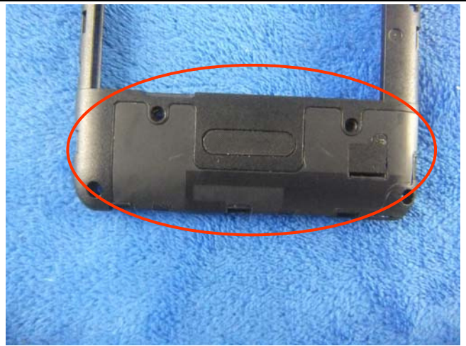
GSM/PCS/UMTS-FDD Antenna View
