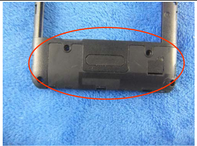
GSM/PCS/UMTS-FDD Antenna View
