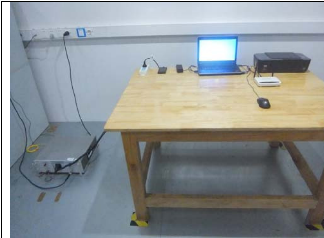
Conducted Emissions Test Setup – Front View
