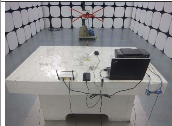
Radiated Emissions Test Setup Below 1GHz
