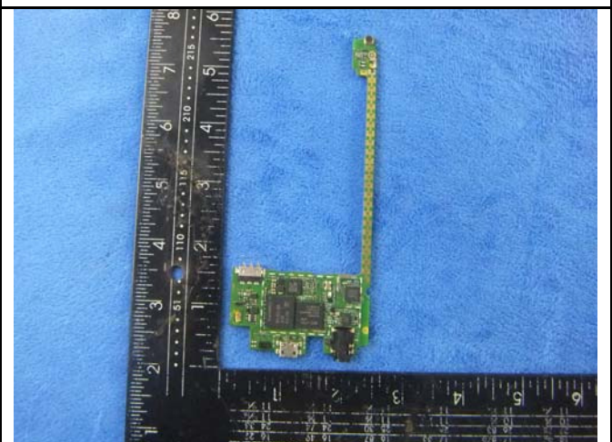
Mainboard without Shielding - Front View
