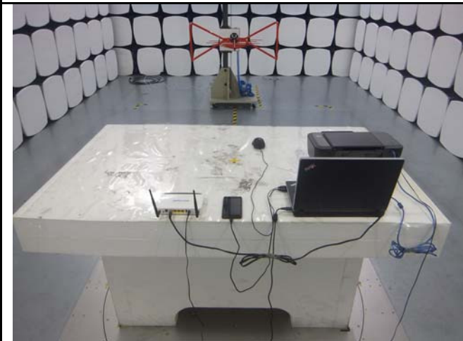
Radiated Emissions Test Setup Below 1GHz
