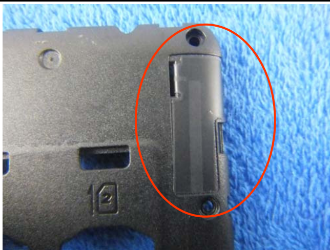
WIFI/BT/BLE/GPS - Antenna View
