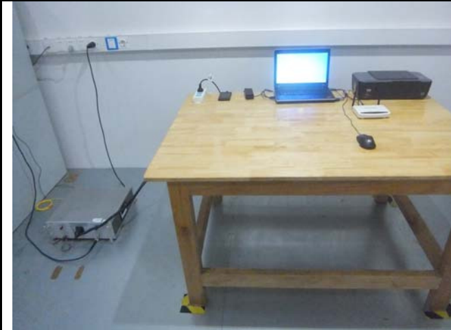
Conducted Emissions Test Setup – Front View
