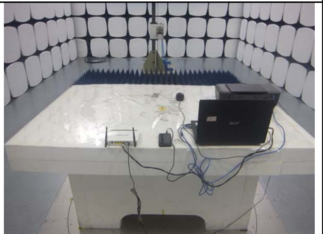
Radiated Emissions Test Setup Above 1GHz
