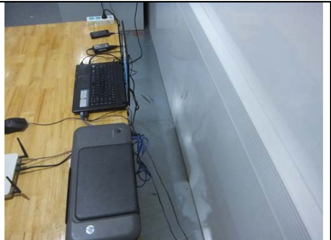
Conducted Emissions Test Setup – Side View
