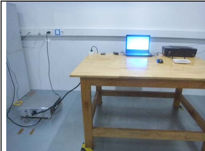
Conducted Emissions Test Setup – Front View
