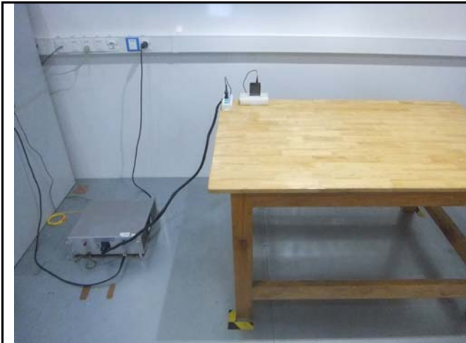
Conducted Emissions Test Setup Front View
