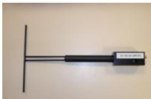
Figure 1 – Satimo COMOSAR Validation Dipole
