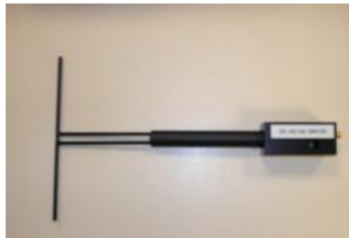
Figure 1 – Satimo COMOSAR Validation Dipole
