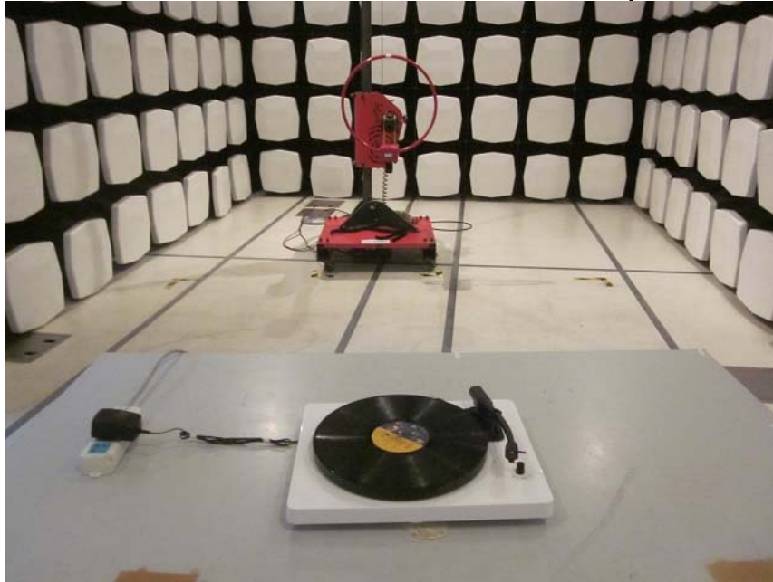
Measurement of Radiated Emission Test Set Up
