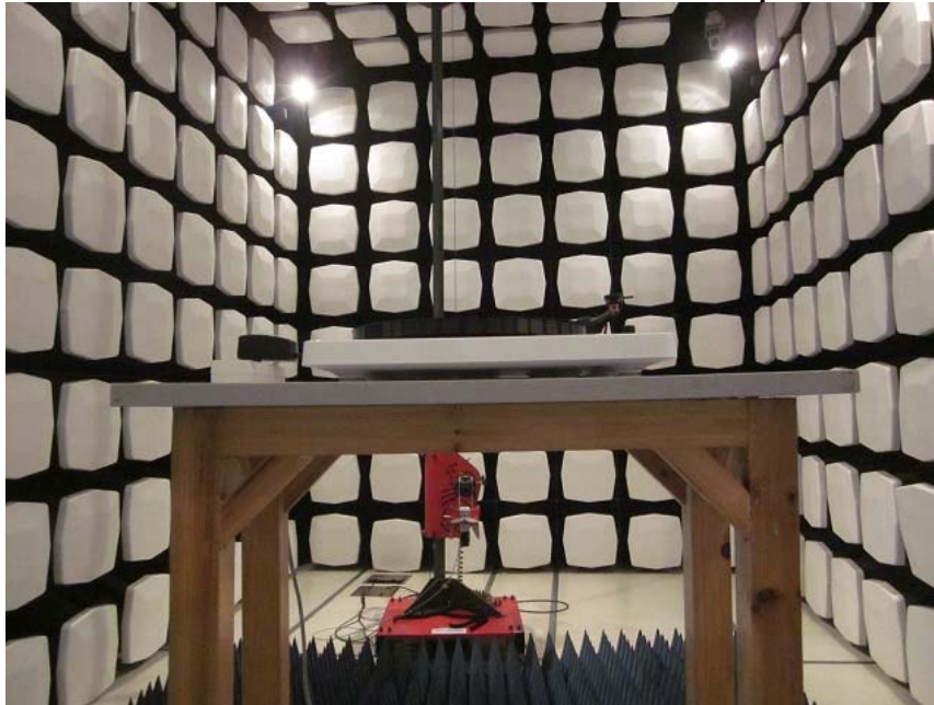
Measurement of Radiated Emission Test Set Up
