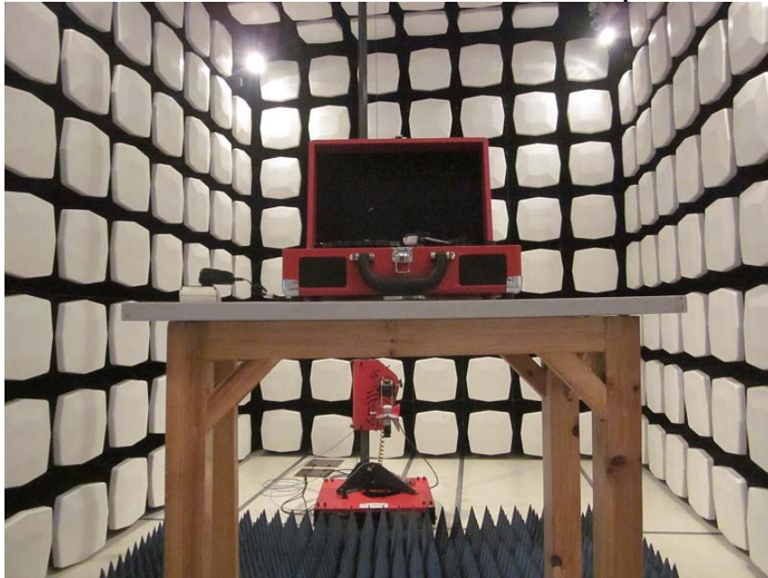
Measurement of Radiated Emission Test Set Up
