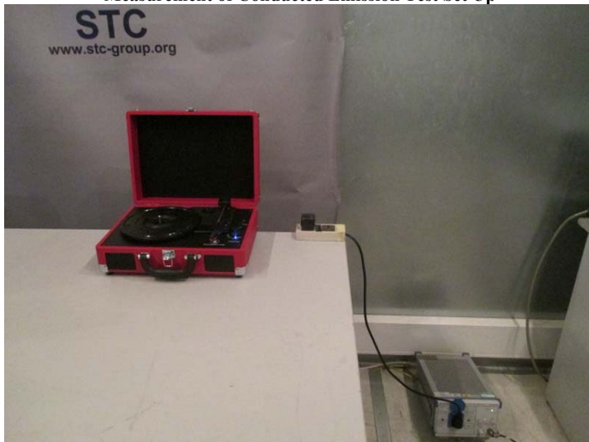
Measurement of Conducted Emission Test Set Up
