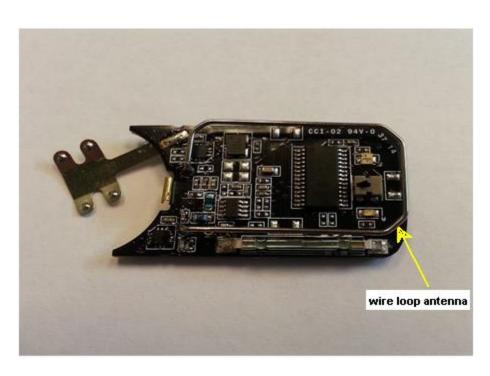
PCB top side and location of "wire loop antenna"
