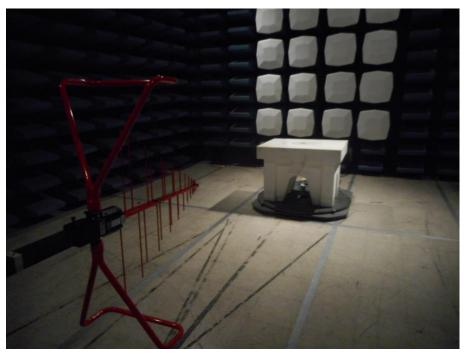
Figure 1: Radiated Spurious Emissions performed at the SAC Test Setup
