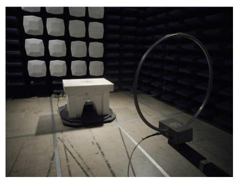
Figure 2: Radiated Spurious Emissions performed at the SAC Test Setup (Below 30MHz)
