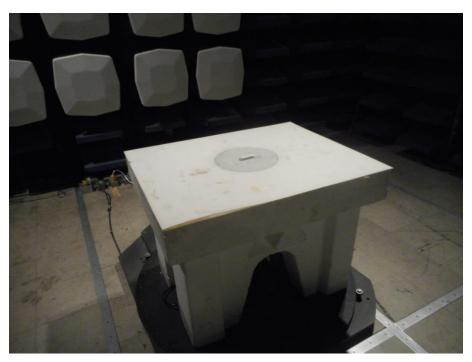
Figure 4: Radiated Spurious Emissions performed at the SAC Test Setup
