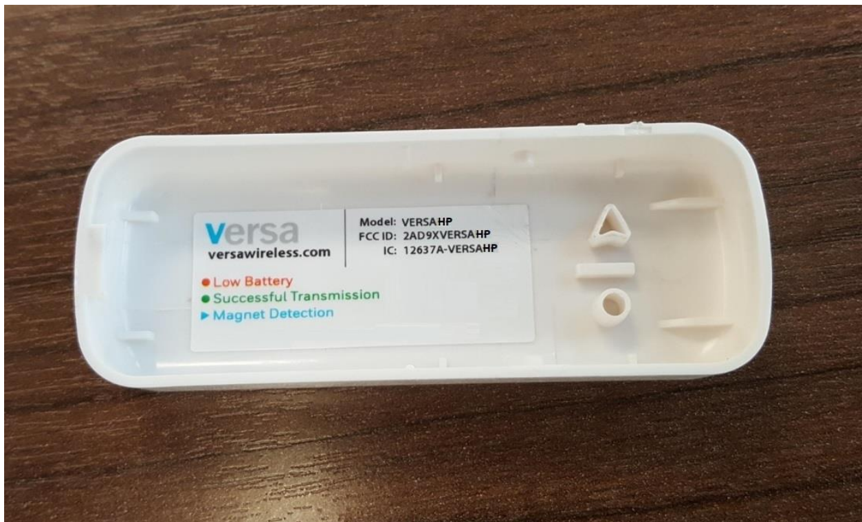
VersaHP Label Location in Housing Lid
