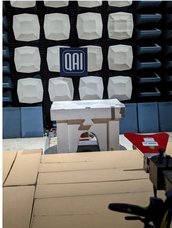
Figure 14: Radiated Emissions from 1 GHz to 6 GHz Setup
