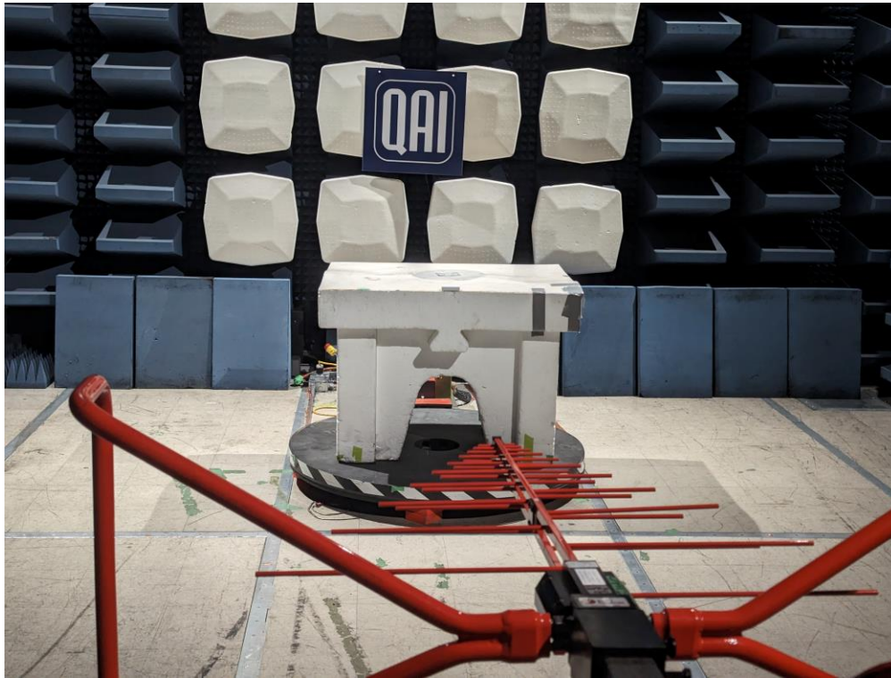
Figure 13: Radiated Emissions From 30 MHz to 1000 MHz Setup
