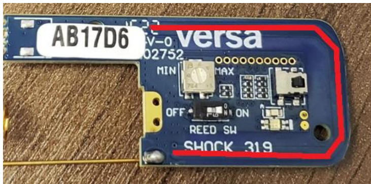
Loop Antenna is a printed trace on the PCB.
