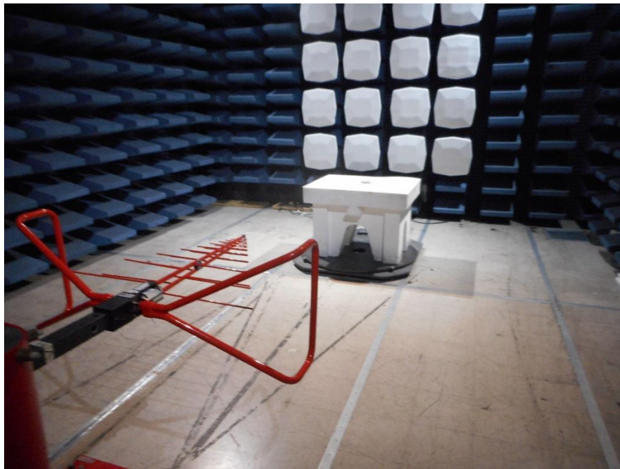
Radiated Emissions 30M – 1 GHz at the 3m SAC
