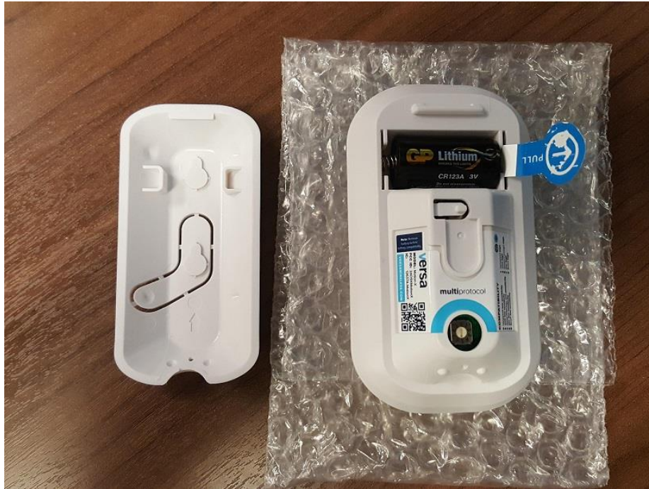
Fig 3 : Motion-X Bottom Side Showing Battery Compartment, Tamper Sw, and Protocol Switch
