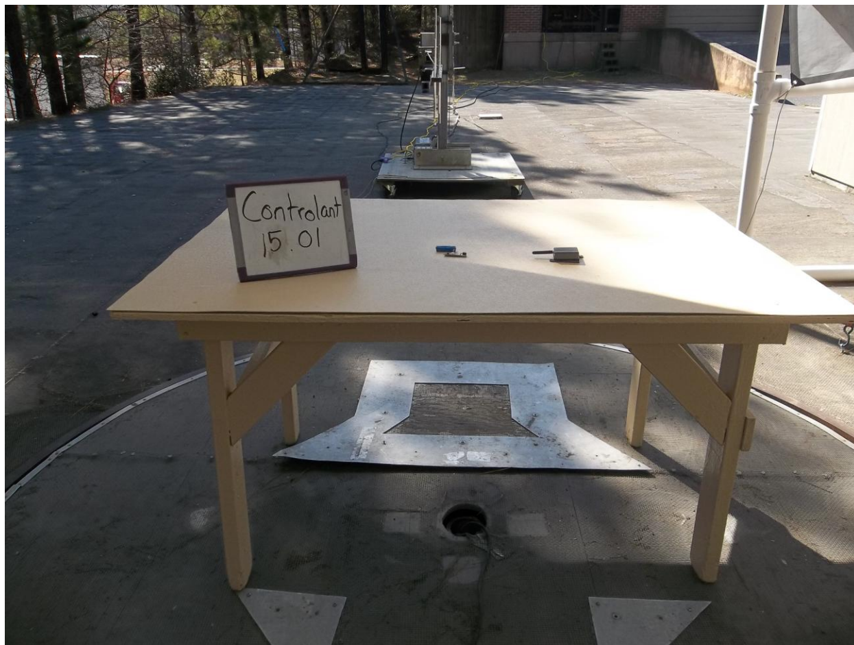
Figure 5. Radiated Emissions Test Setup, 200 MHz to 1GHz, Back
