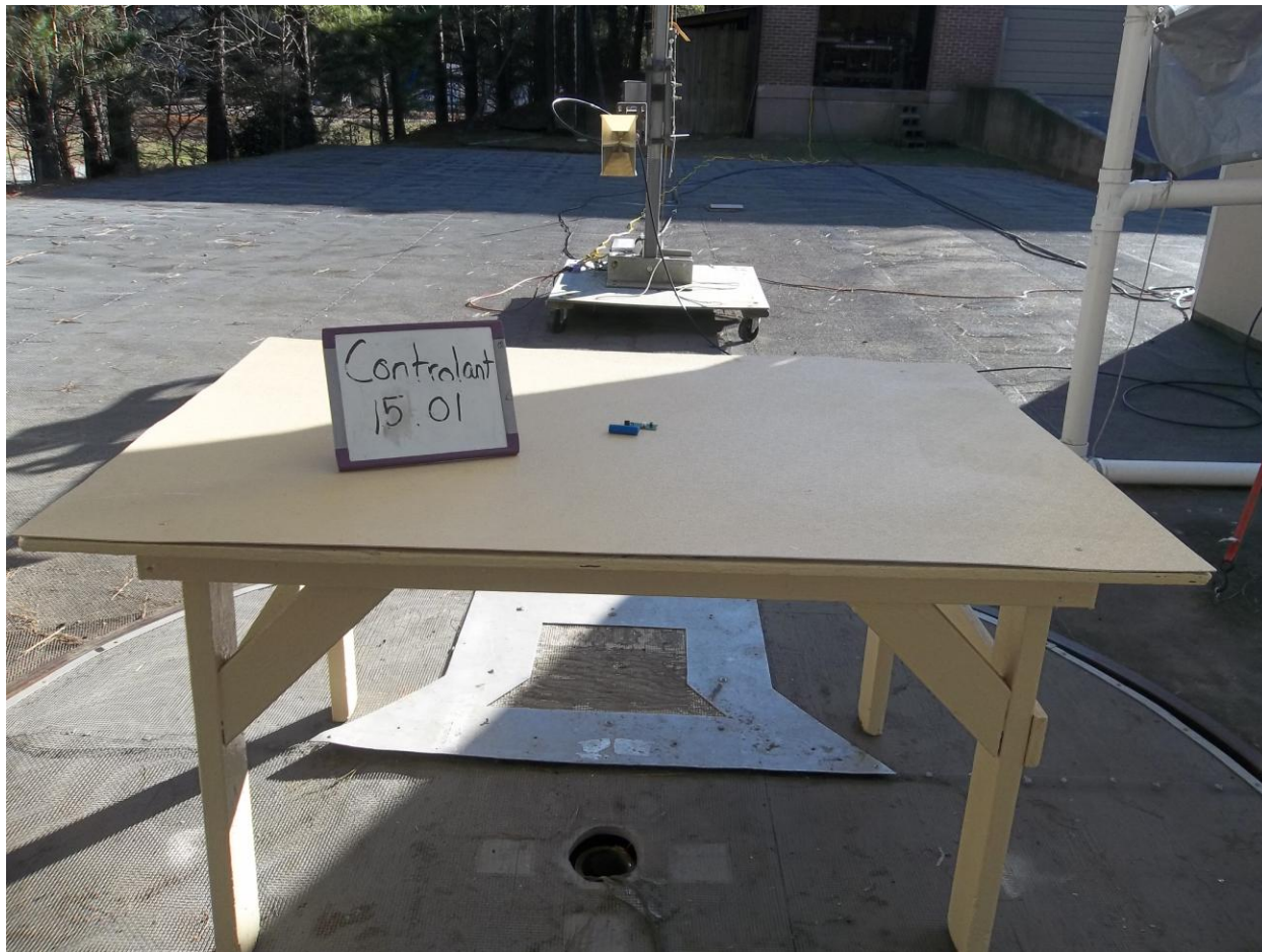
Figure 8. Radiated Emissions Test Setup, above 1 GHz, Back (Harmonic Measurements)
