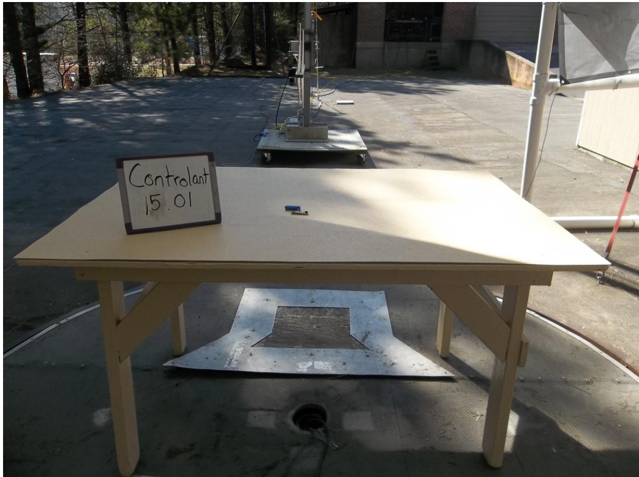
Figure 6. Radiated Emissions Test Setup, 200 MHz to 1GHz, Back (Fundamental Measurements)
