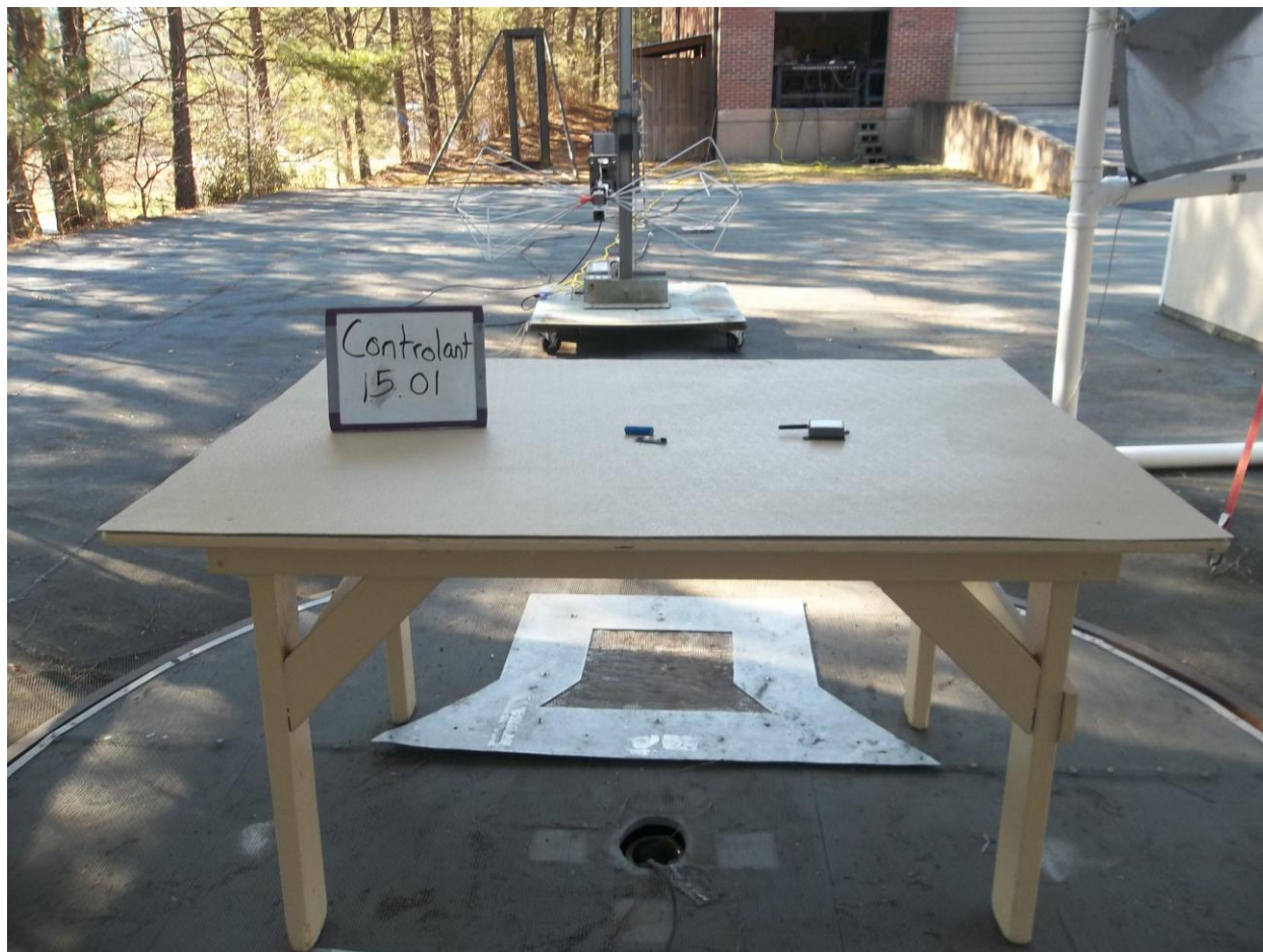
Figure 4. Radiated Emissions Test Setup, 30 MHz to 200 MHz, Back
