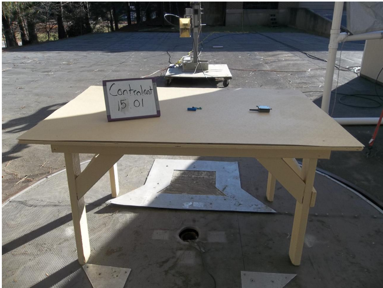
Figure 7. Radiated Emissions Test Setup, above 1 GHz, Back
