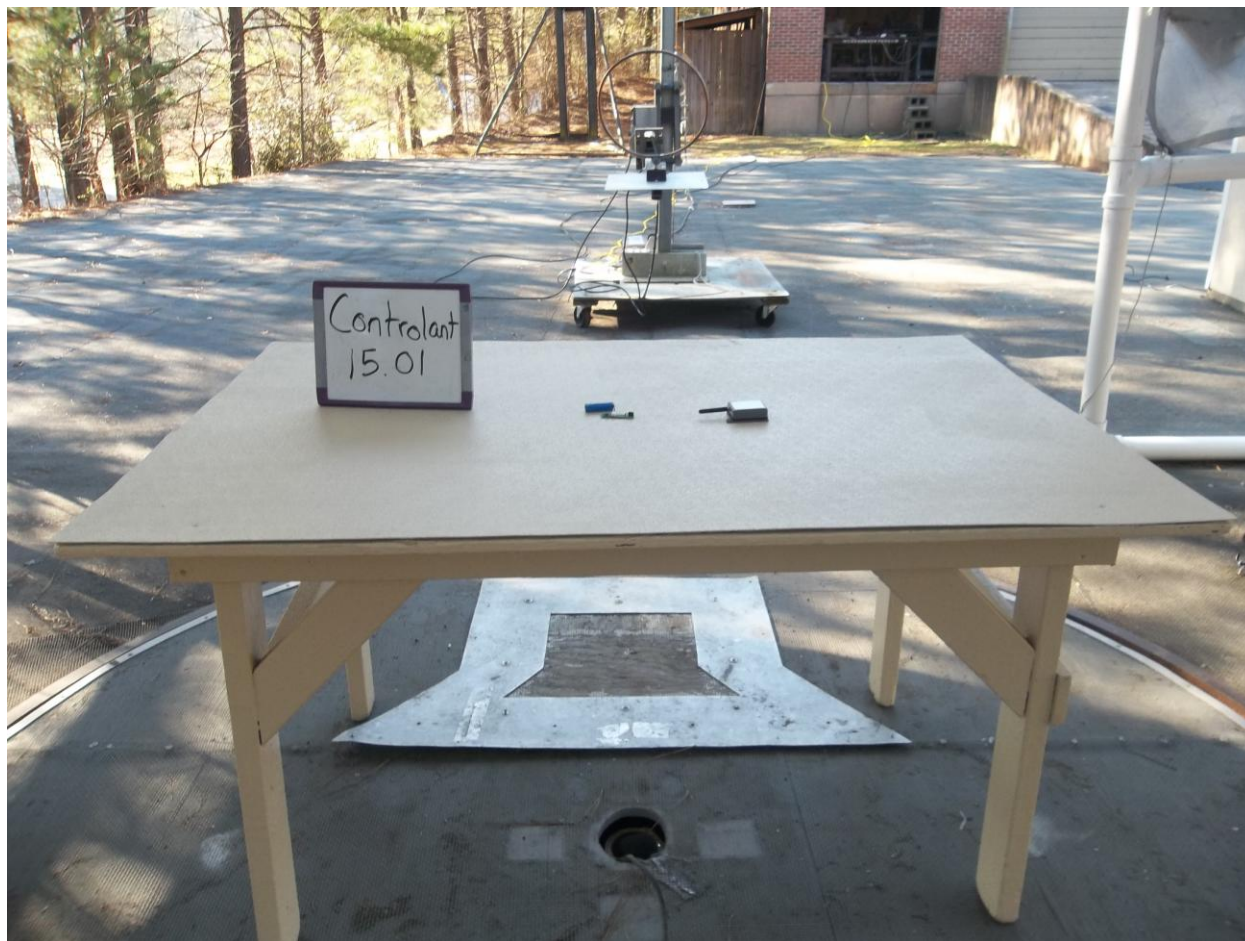
Figure 3. Radiated Emissions Test Setup, .15 MHz to 30 MHz, Back
