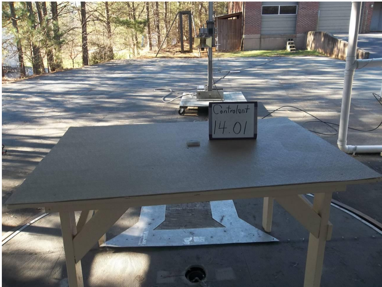
Figure 7. Radiated Emission Test Setup, above 1 GHz, Back
