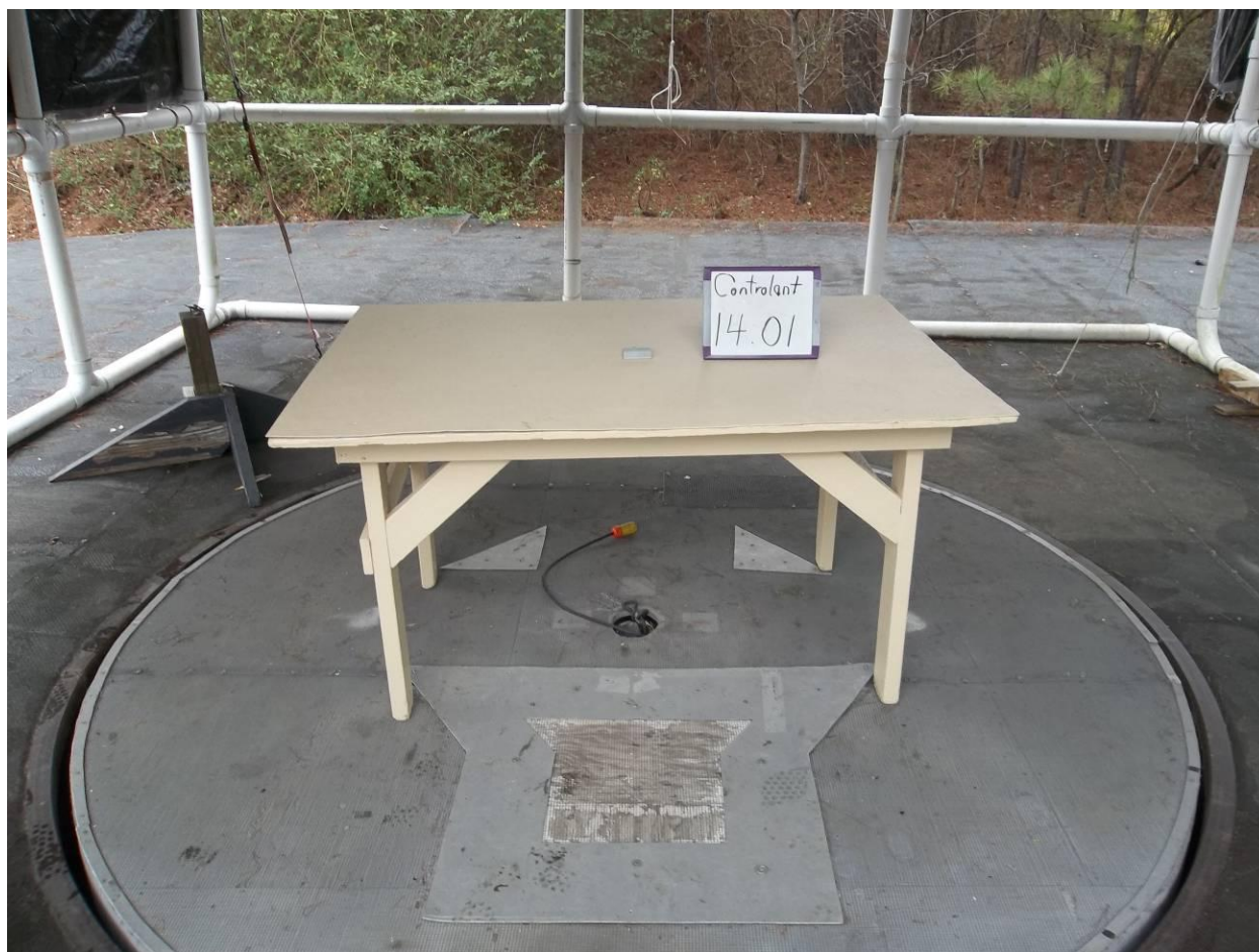
Figure 1. Radiated Emissions Test Setup, Front - for Normal Use Mode
