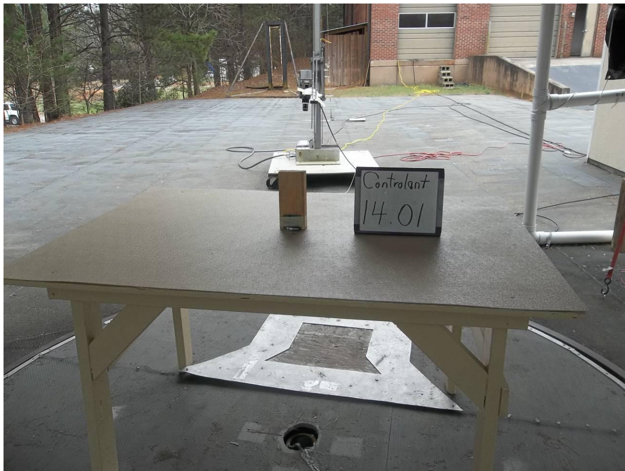
Figure 8. Radiated Emissions Test Setup, 200 MHz to 1GHz, Back for Continuous Transmission (Fundamental Measurement)
