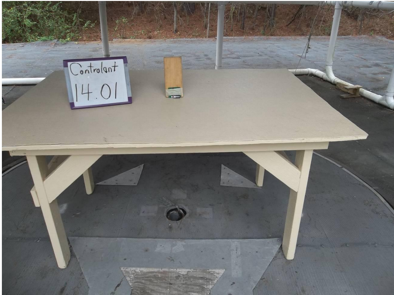
Figure 2. Radiated Emissions Test Setup, Front - for Continuous Transmission Measurements (Fundamental & Harmonic)
