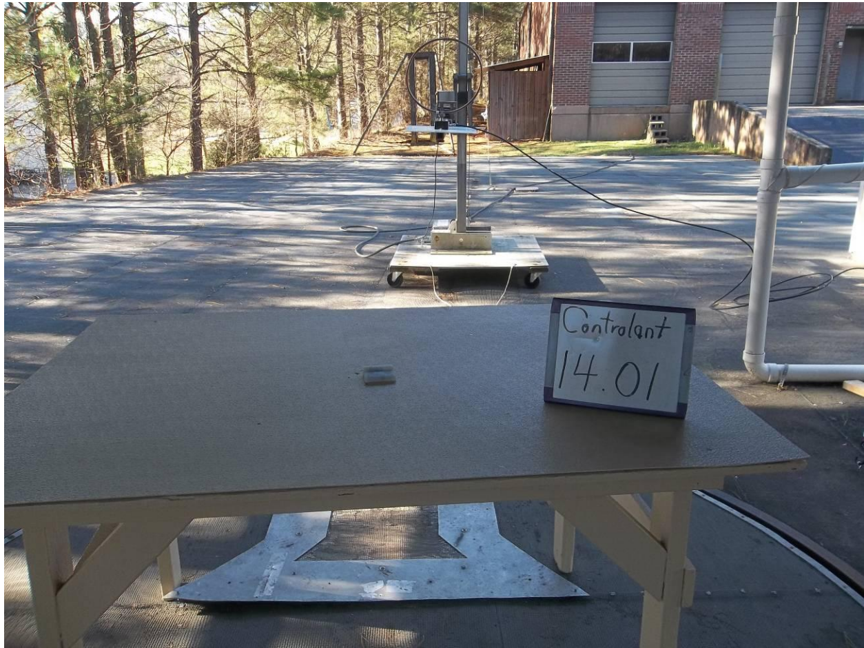
Figure 4. Radiated Emissions Test Setup, 0.15 MHz to 30 MHz, Back
