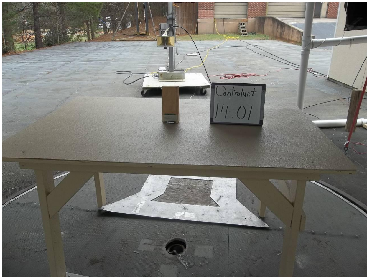
Figure 9. Radiated Emission Test Setup, above 1 GHz, Back for Continuous Transmission (Harmonic Measurements)
