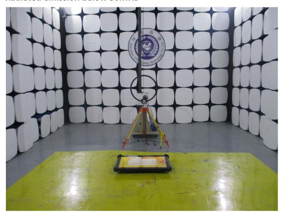
Radiated emission 30MHz to 1GHz
