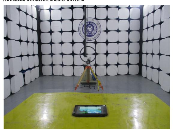
Radiated emission 30MHz to 1GHz
