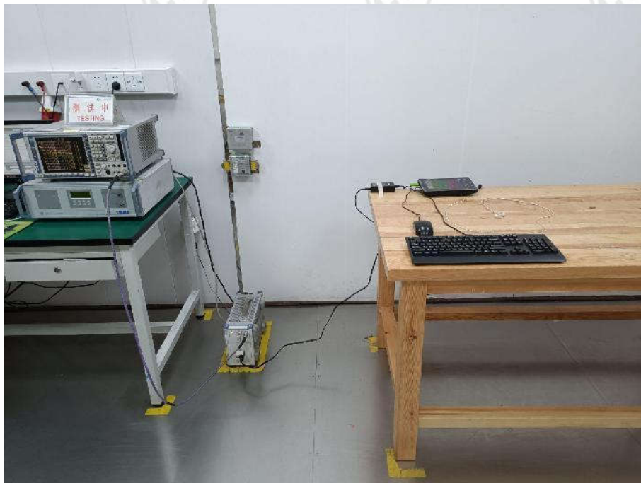
Conducted Emissions Test Setup
