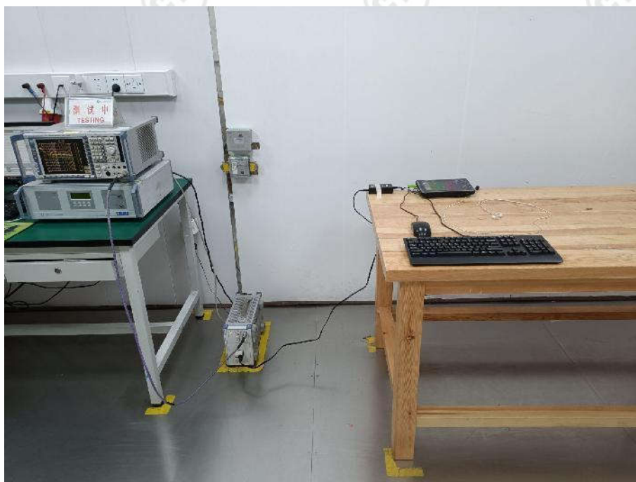
Conducted Emissions Test Setup
