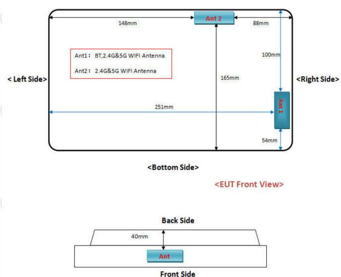
Note:1)Per KDB 616217, because the diagonal Length is >200mm, it is considered a "tablet" device and need to test 0mm 1g Body SAR.
