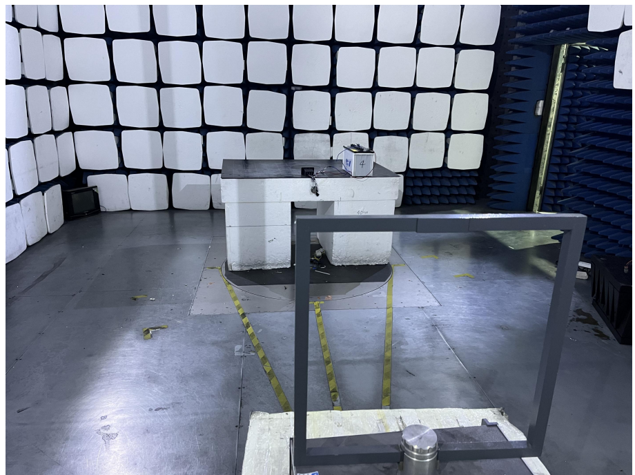
Radiation Emission Test Setup (Below 30MHz)
