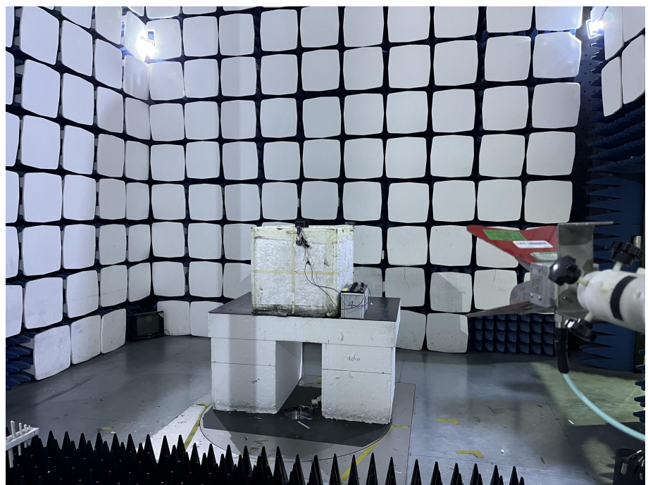
Radiation Emission Test Setup (1GHz to 18GHz)
