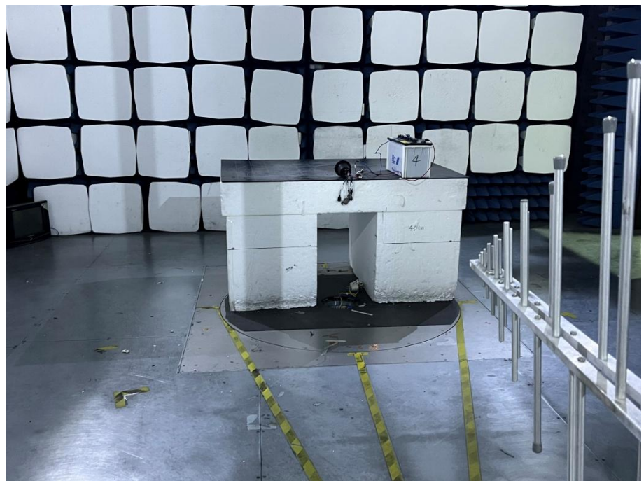
Radiation Emission Test Setup (30MHz to 1GHz)
