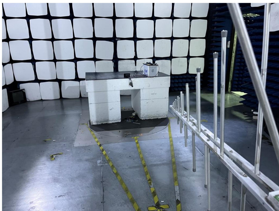
Radiation Emission Test Setup (30MHz to 1GHz)
