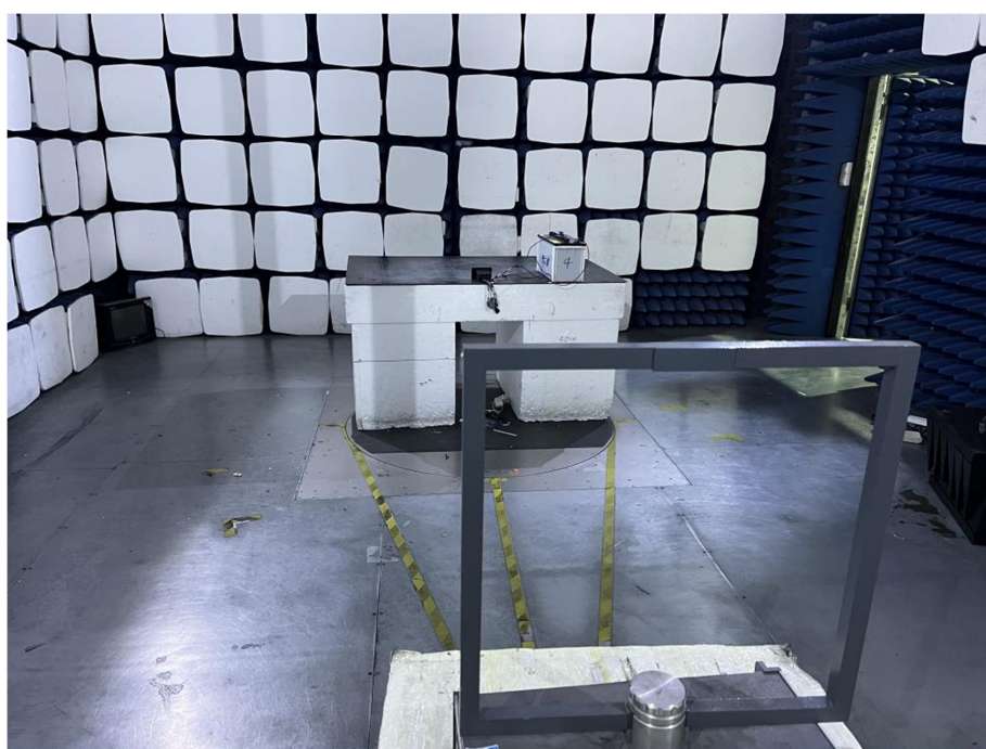
Radiation Emission Test Setup (Below 30MHz)
