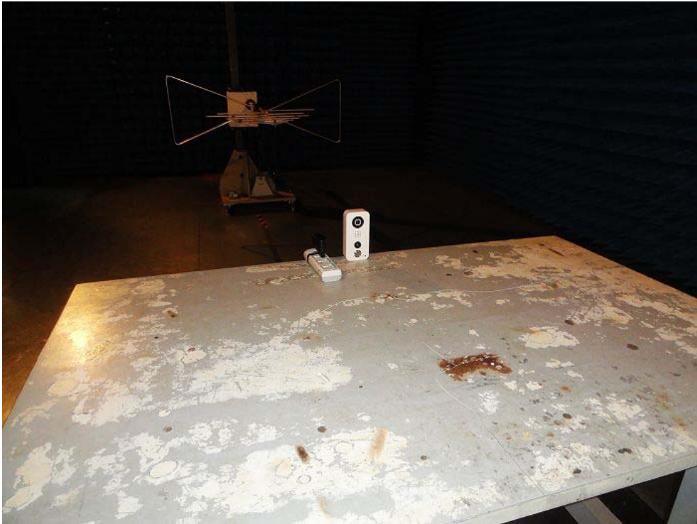
Radiated emission test view
