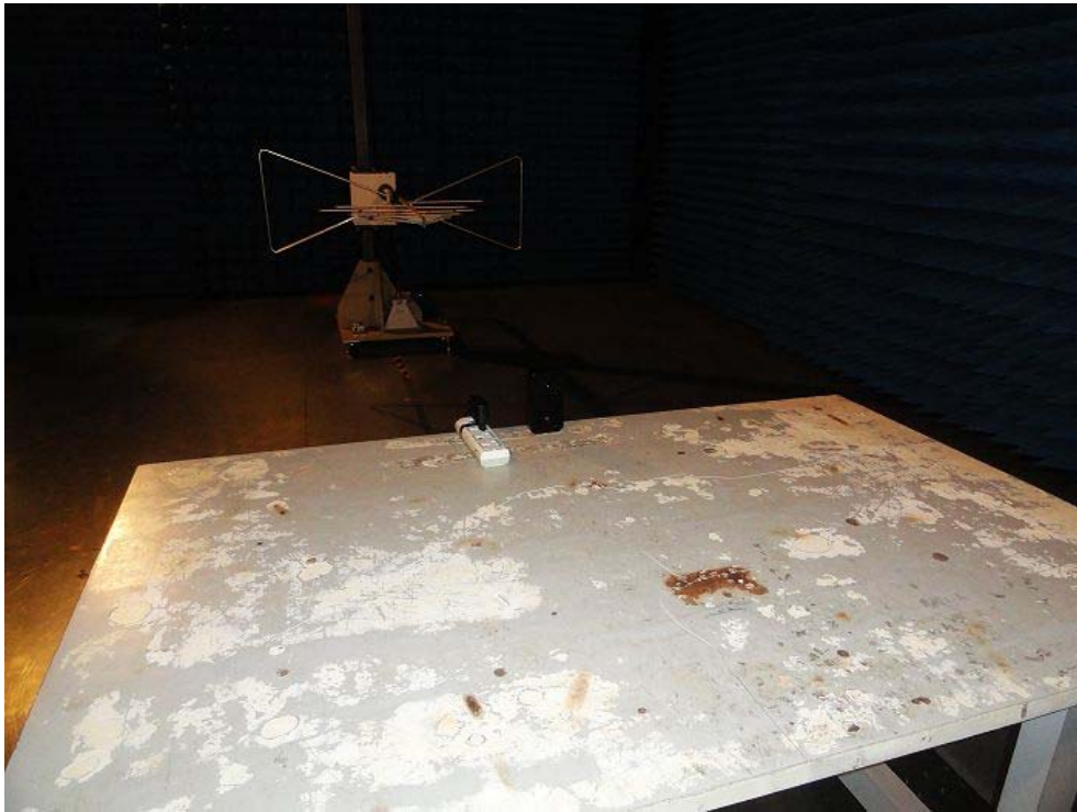
Radiated Emission Test Setup:
