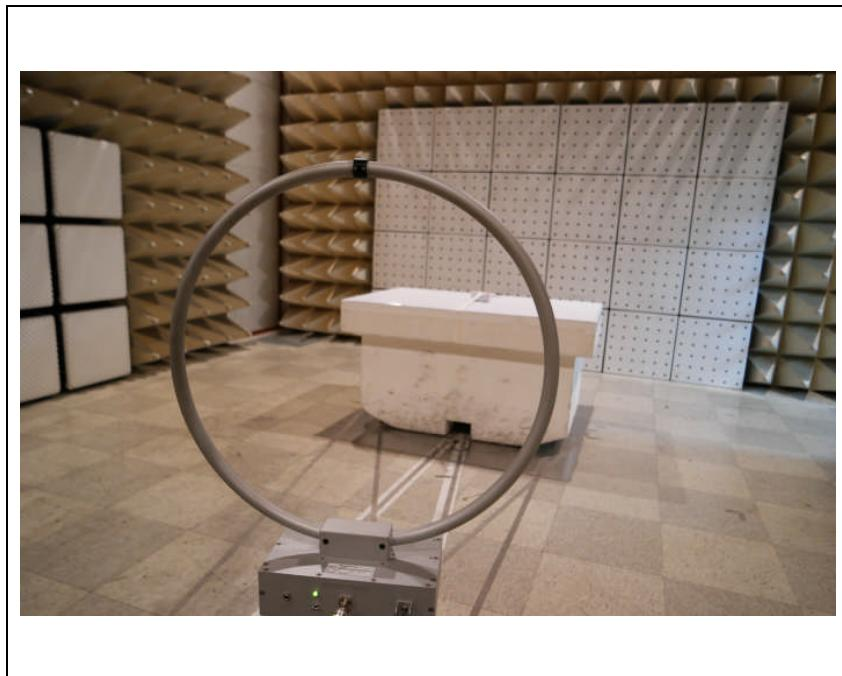
**C. Photo of Test setup (30 MHz ~ 1 GHz)**
