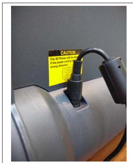
2. Plug the power supply output plug (24V DC) to the 3D Printer power input socket
