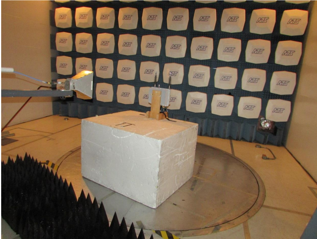
Radiated Emissions Setup – 10GHz to 18GHz
