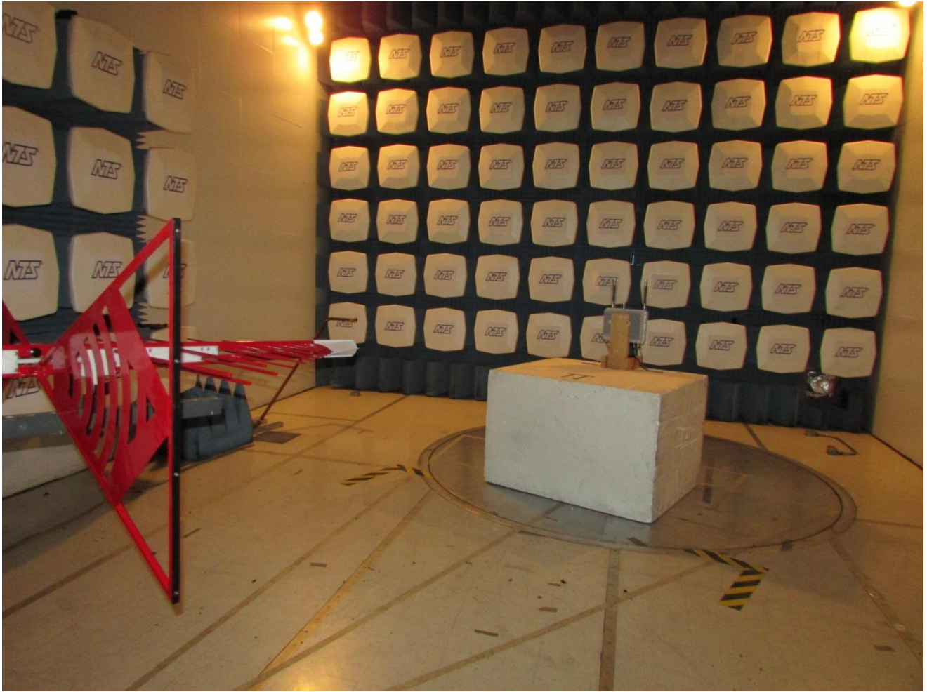
Radiated Emissions Setup – 30MHz to 1GHz
