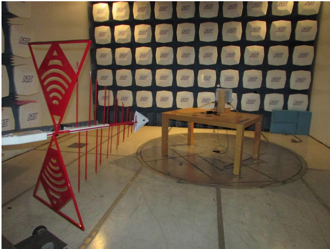
Radiated Emissions Setup – 30MHz to 1GHz
