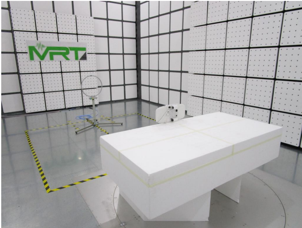
Description: Galtronics Omni Antenna Radiated Emission Test Setup for 30MHz ~ 1GHz
