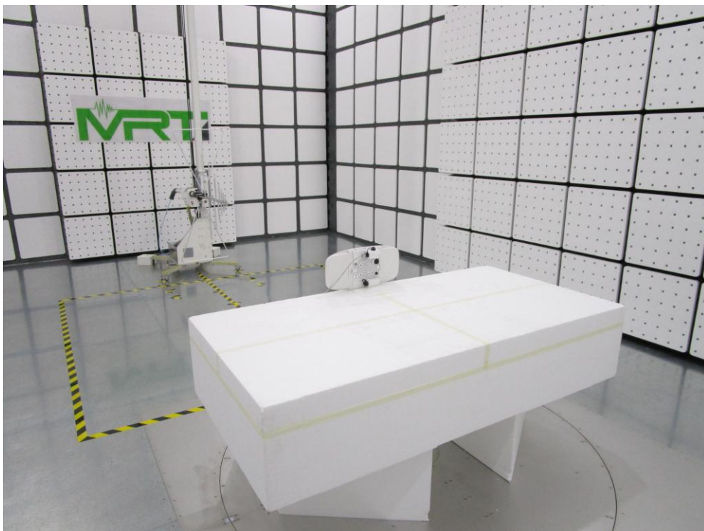
Description: Galtronics Omni Antenna Radiated Emission Test Setup for 30MHz ~ 1GHz
