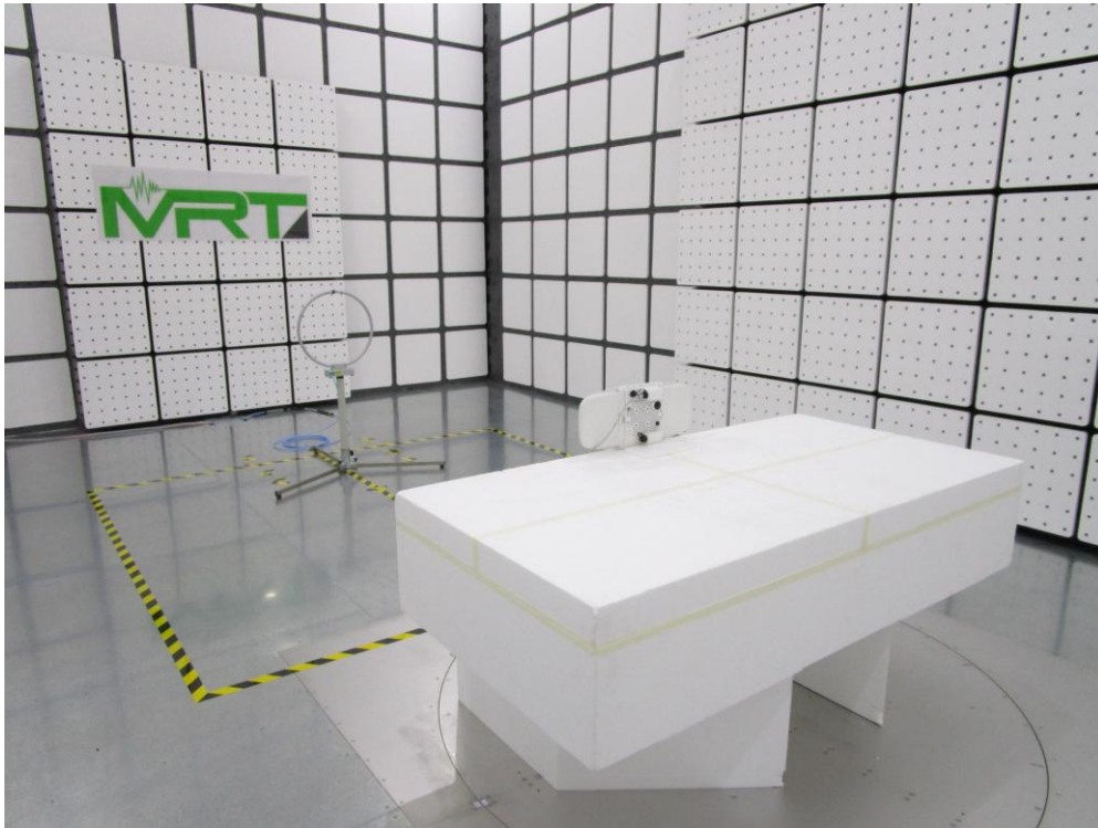
Description: Galtronics Directional Antenna Radiated Emission Test Setup for 30MHz ~ 1GHz
