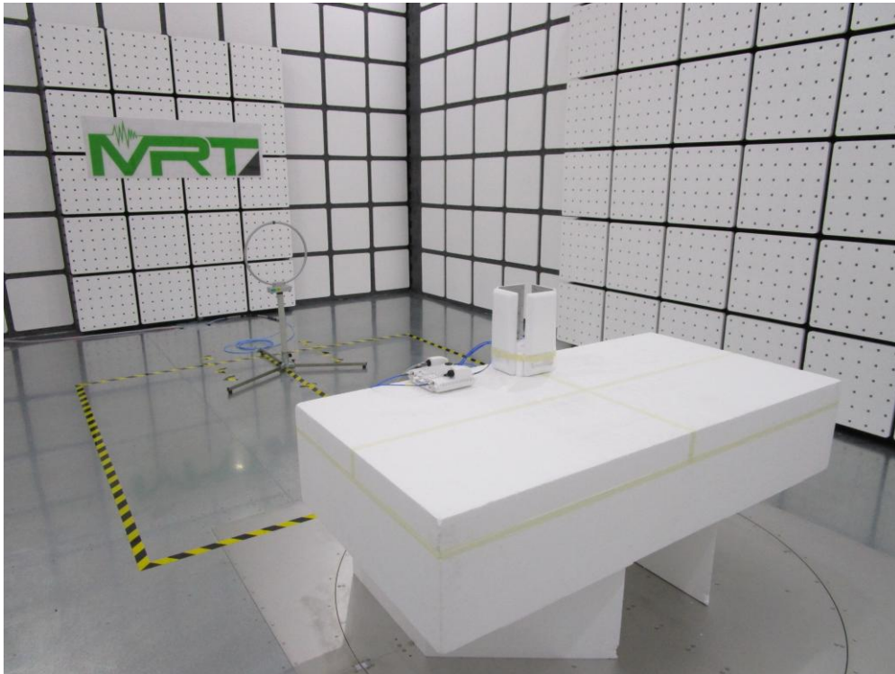
Description: Sector-Antenna 1356.17.0011 Antenna Radiated Emission Test Setup for 30MHz ~ 1GHz
