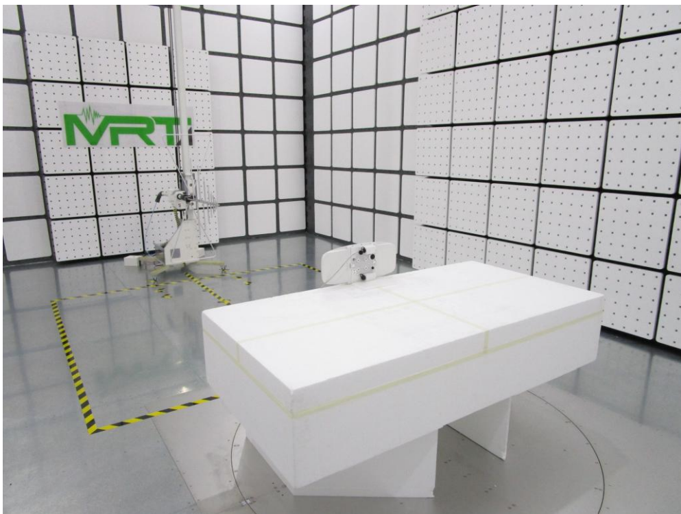
Description: Galtronics Directional Antenna Radiated Emission Test Setup for 30MHz ~ 1GHz
