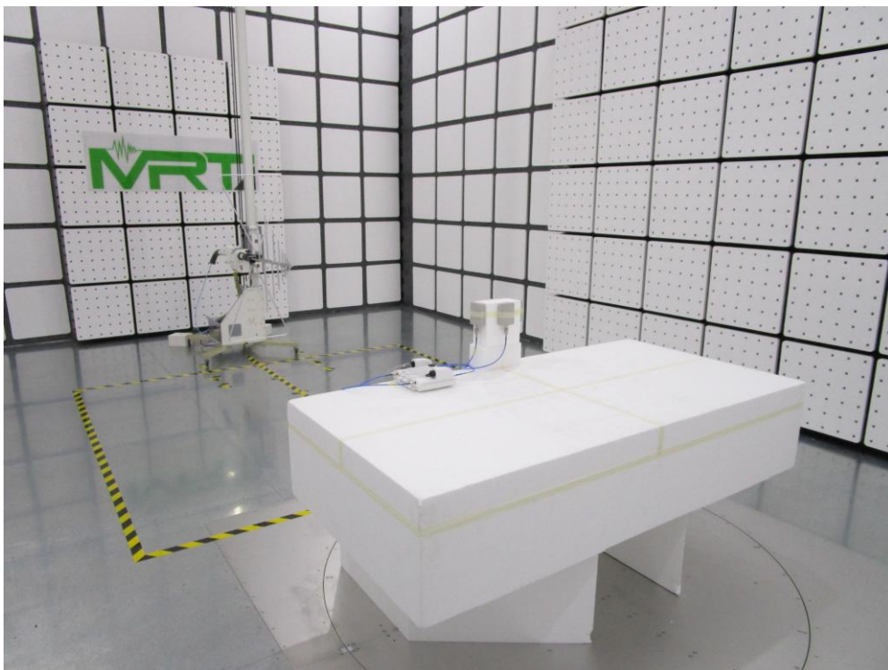
Description: Directional Antenna 1356.17.0077 Radiated Emission Test Setup for 30MHz ~ 1GHz
