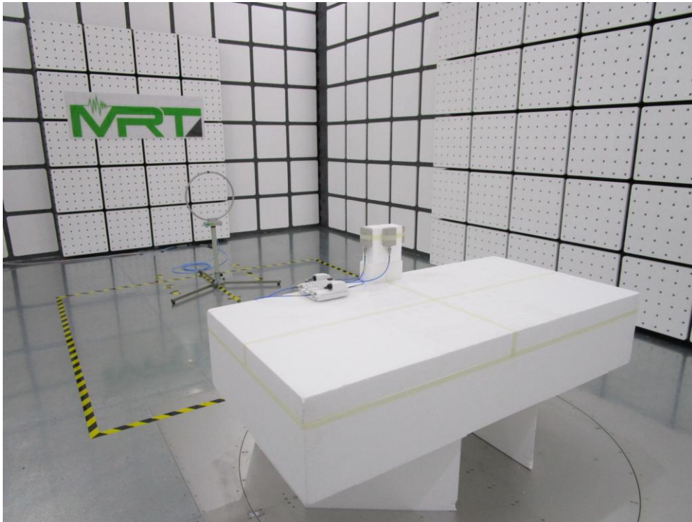
Description: Directional Antenna 1356.17.0077 Radiated Emission Test Setup for 30MHz ~ 1GHz
