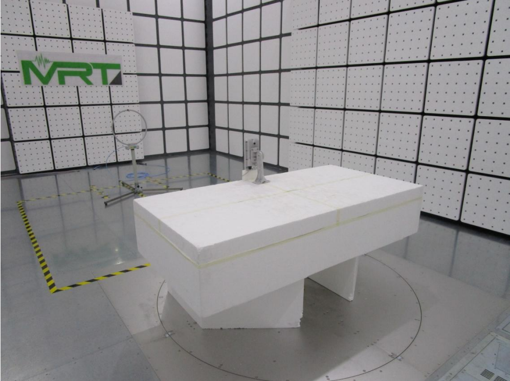
Description: AC220 Wi-Fi AP OD external antenna US Radiated Emission Test Setup for 9kHz ~ 30MHz
