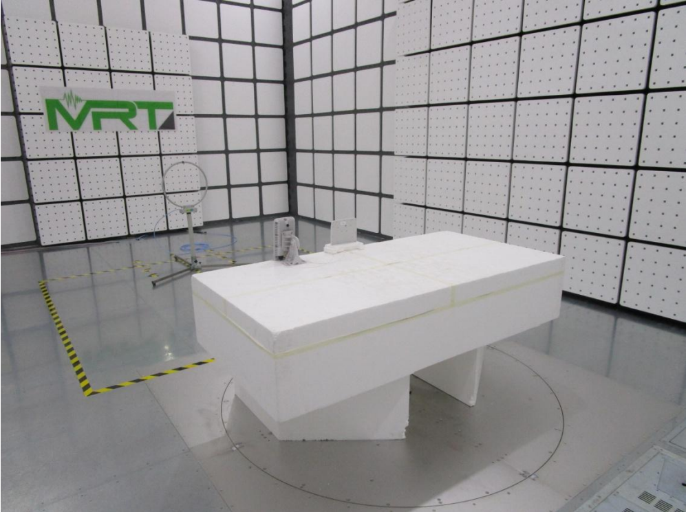
Description: AC220 Wi-Fi AP OD external antenna US Radiated Emission Test Setup for 9kHz ~ 30MHz
