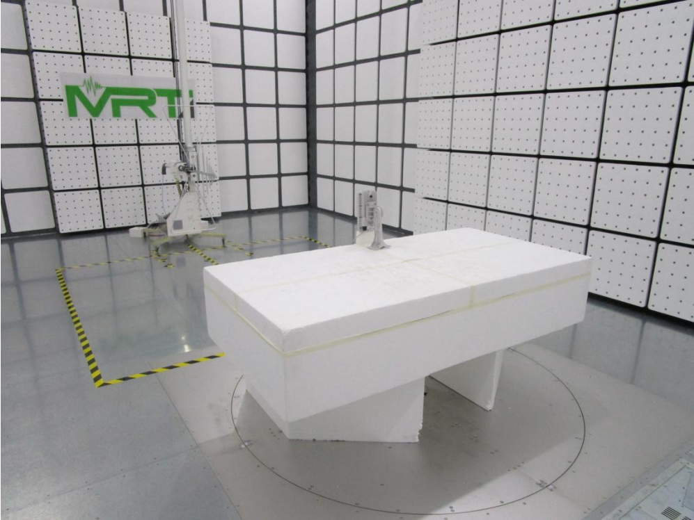
Description: AC220 Wi-Fi AP OD directional antenna US Radiated Emission Test Setup for 30MHz ~ 1GHz
