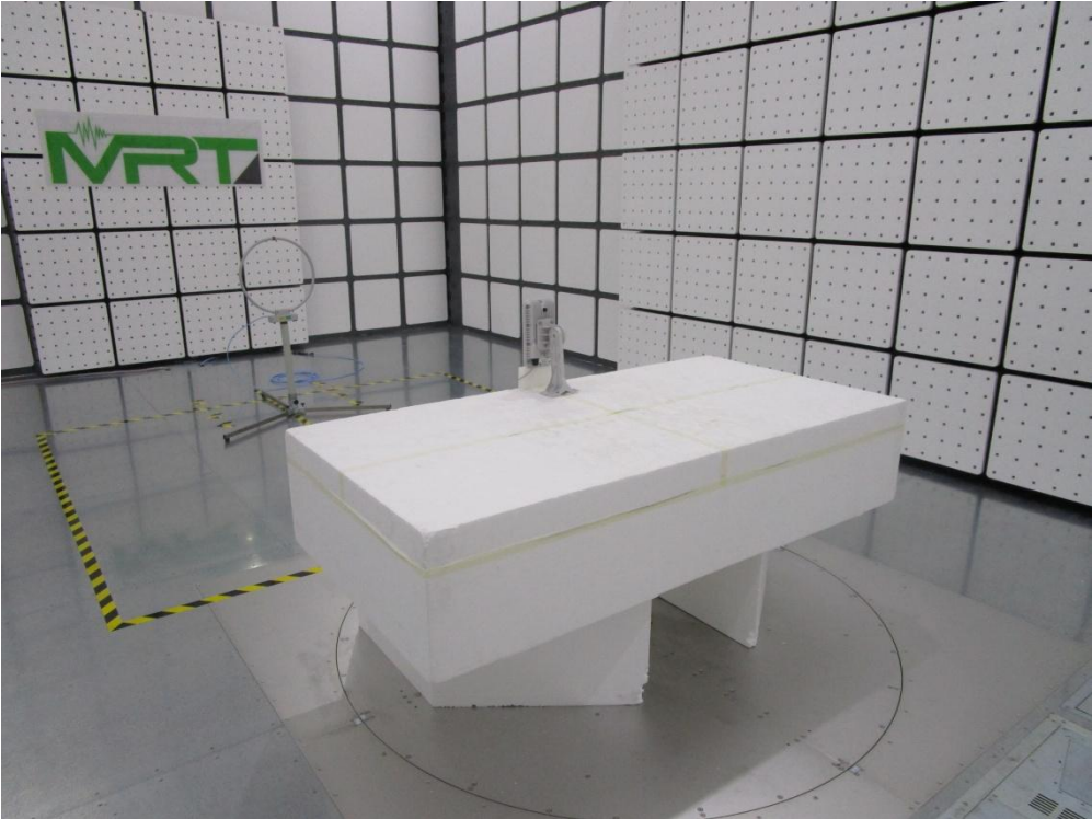
Description: AC220 Wi-Fi AP OD directional antenna US Radiated Emission Test Setup for 30MHz ~ 1GHz
