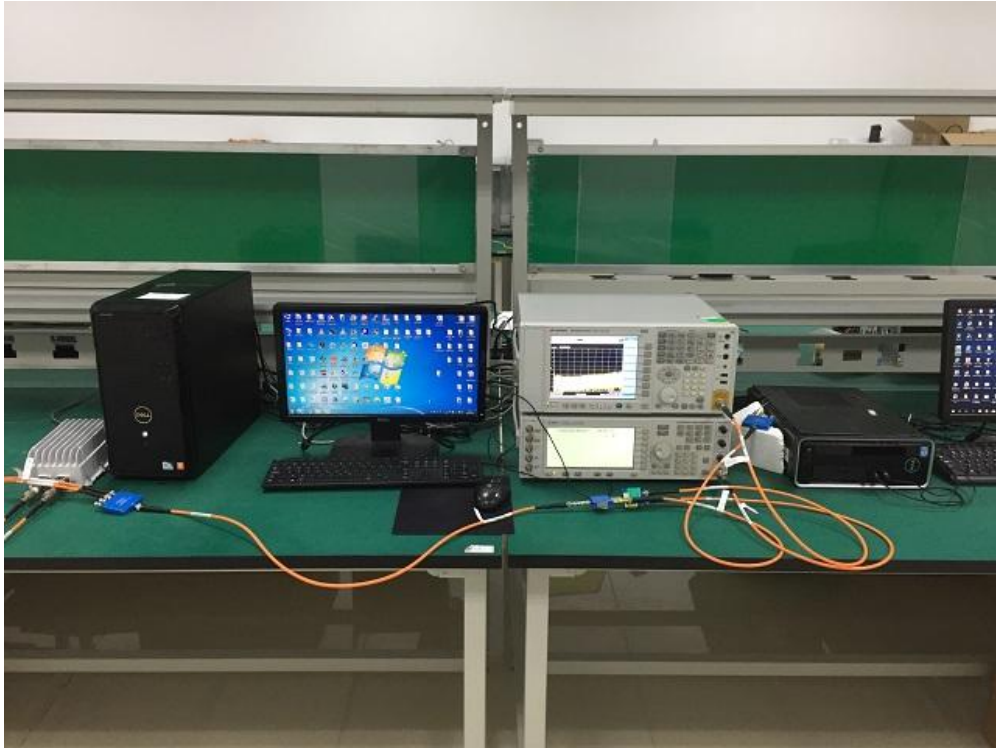
Description: DFS Test Setup
