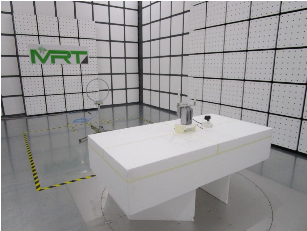
Description: WiFi Dual-band Omni Directional Antenna Radiated Emission Test Setup for 30MHz ~ 1GHz
