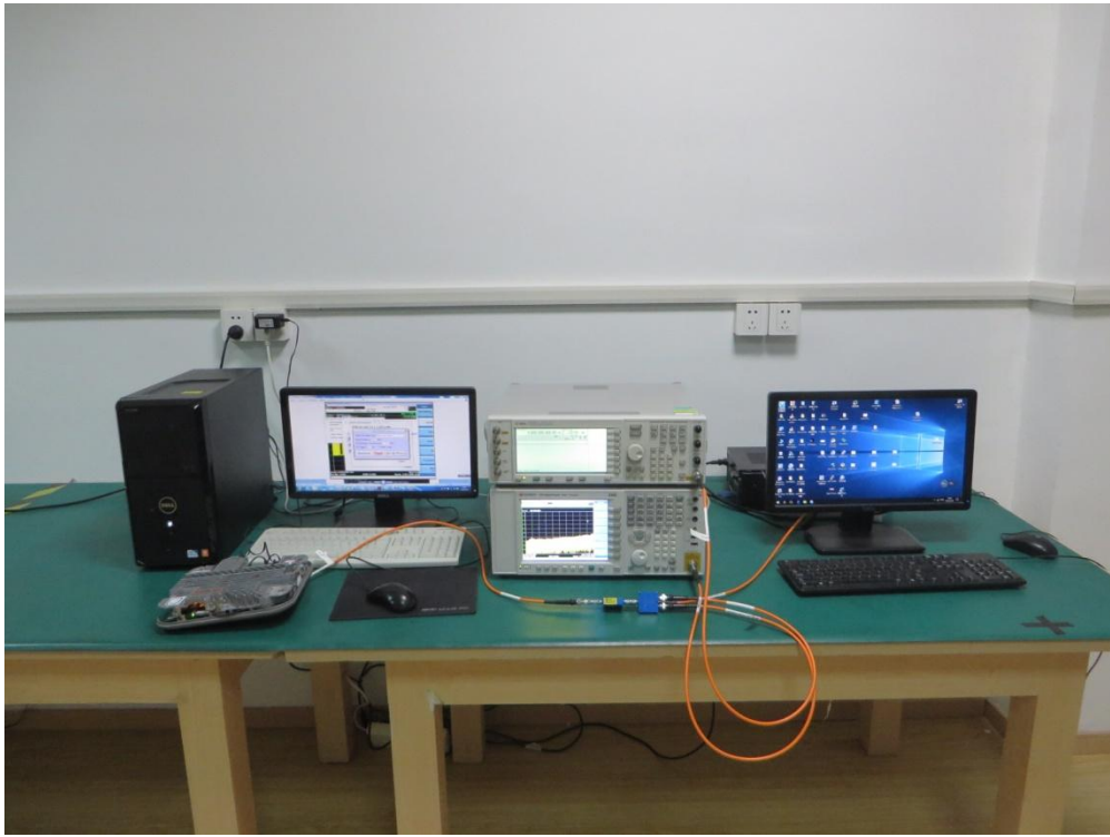
Description: DFS Test Setup
